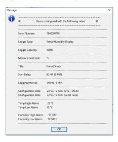
Click OK and disconnect logger from the USB port of PC
